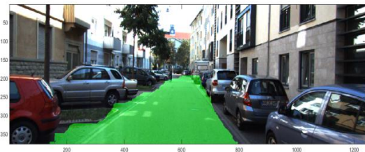
Fig 4 Typical road detection results of the proposed method
